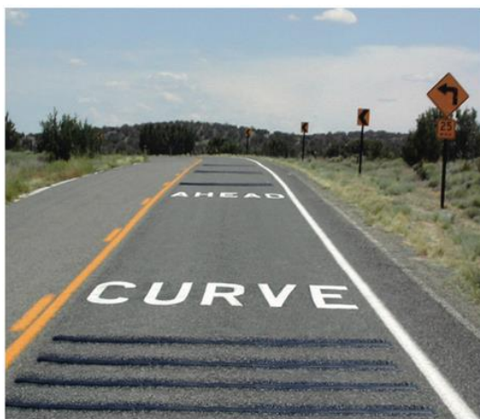
Above, left: "CURVE AHEAD" paired with transverse rumble strips. Right: "SLOW" and arrow.
