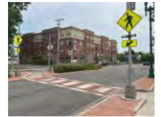
Rectangular rapid flashing beacons
