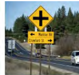
Oversized advance intersection warning signs
