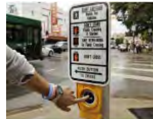
Accessible pedestrian signals
